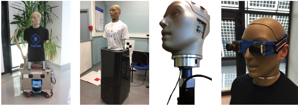
Figure 3.2: From left to right: TWO!EARS binaural robots, consisting of a KEMAR HATS and a mobile platform; motorisation of the KEMAR head; stereoscopic setup.
