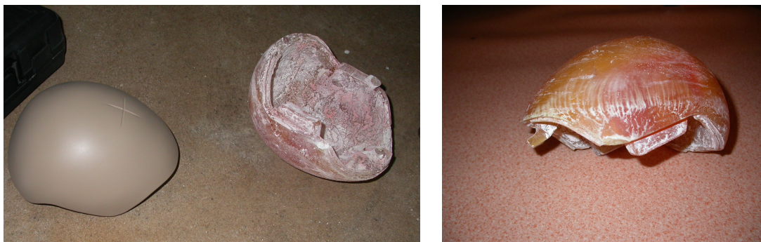
Figure 8.3: Molding of another cover for the KEMAR head, which could support a stereo rig.
