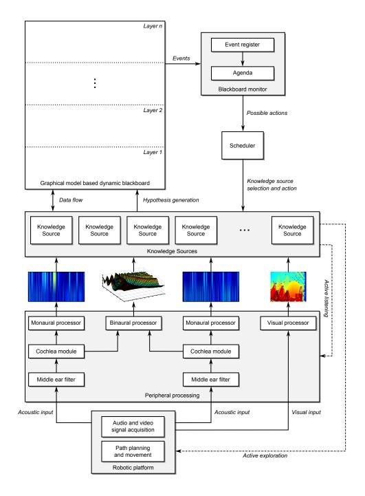
Figure 2.1: Overview of the general Two!EARS software architecture.
