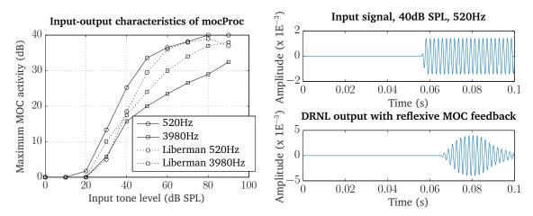
**Figure 4.14:** Left panel: input-output characteristics of the MOC processor for on-frequency tone stimulus at 520 and 3980Hz. The data set of Liberman (1988), scaled as in the work of Clark *et al.* (2012), is also shown for comparison. Right panel: DRNL processor output (bottom) from a 50-ms tone at 40dB SPL and 520Hz (top), with the reflexive MOC feedback operating.
