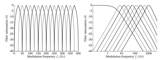
**Figure 4.15:** Transfer functions of 15 linearly-scaled (left panel) and 9 logarithmically-scaled (right panel) modulation filters.
