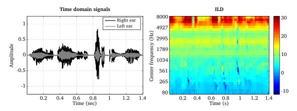
**Figure 4.21:** Binaural speech signal (left panel) and the estimated ILD in dB shown as a function of time frames and frequency channels.
