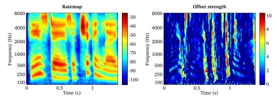
**Figure 4.11:** Ratemap representation (left panel) of speech and the corresponding offset strength in dB (right panel).
