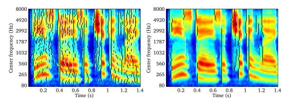
**Figure 4.12:** Detected onsets and offsets indicated by the black and white vertical bars. The left panels shows all onset and offset events, whereas the right panel applies temporal and across-frequency constraints in order to retain the most salient onset and offset events.
