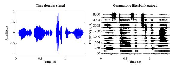
**Figure 4.2:** Time domain signal (left panel) and the corresponding output of the gammatone processor consisting of 16 auditory filters spaced between 80 and 8000 Hz (right panel).
