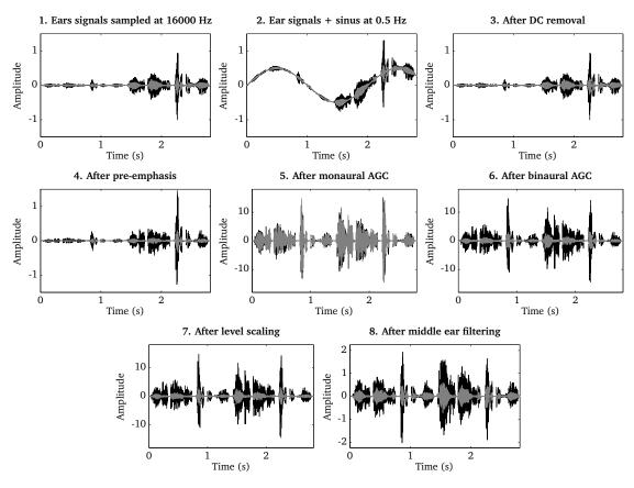
Figure 4.1: Illustration of the individual pre-processing steps. 1) Ear signals consisting of two sentences recorded at different levels, 2) ear signals mixed with a 0.5 Hz humming 3), ear signals after DC removal filter, 4) influence of pre-emphasis filter, 5) monaural RMS normalization, 6) binaural RMS normalization, 7) level scaling and 8) middle ear filtering.
