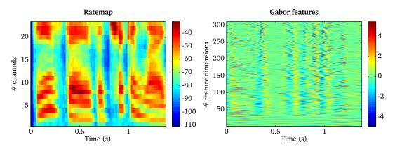
**Figure 4.18:** Ratemap representation of a speech signal (left panel) and the corresponding output of the Gabor feature processor (right panel).
