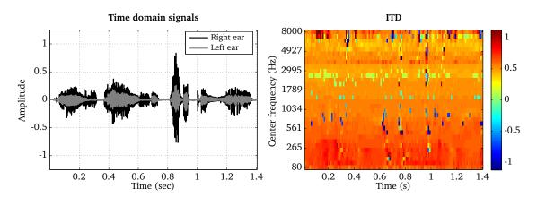
**Figure 4.20:** Binaural speech signal (left panel) and the estimated ITD in ms shown as a function of time frames and frequency channels.
