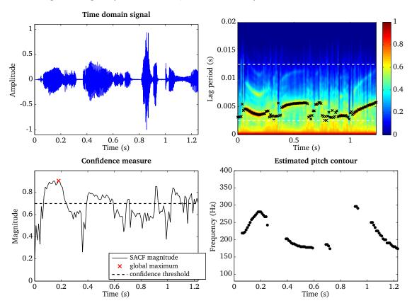
**Figure 4.13:** Time domain signal (top left panel) and the corresponding SACF (top right panel). The confidence measure based on the SACF magnitude is used to select reliable pitch estimates (bottom left panel). The final pitch estimate is post-processed by a median filter (bottom right panel).
