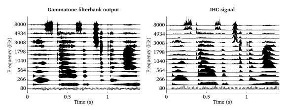
Figure 4.5: Illustration of the envelope extraction processor. BM output (left panel) and the corresponding IHC model output using ihc\_method = 'dau' (right panel).
