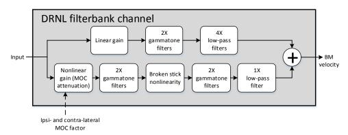
**Figure 4.3:** DRNL filterbank channel structure, following the CASP model specification (Jepsen *et al.*, 2008) as default, with an additional nonlinear gain stage to receive feedback.
