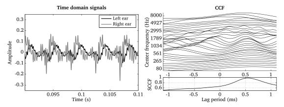
**Figure 4.19:** Left and right ear signals shown for one time frame of 20 ms duration (left panel) and the corresponding CCF (right panel). The SCCF summarizes the CCF across all auditory channels (bottom right panel).
