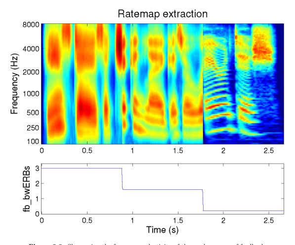
Figure 2.3: Sharpening the frequency selectivity of the ear by means of feedback
