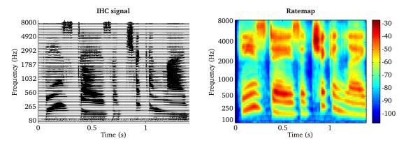
**Figure 4.8:** IHC representation of s speech signal using 64 auditory filters (left panel) and the corresponding ratemap representation (right panel).
