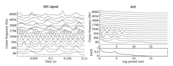
**Figure 4.7:** IHC representation of a speech signal shown for one time frame of 20 ms duration (left panel) and the corresponding ACF (right panel). The SACF summarizes the ACF across all frequency channels (bottom right panel).
