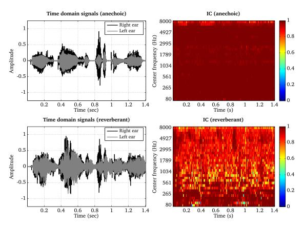
**Figure 4.22:** Time domain signals and the corresponding interaural coherence as a function of time frames and frequency channels estimated for a speech signal in anechoic and reverberant conditions. Anechoic speech (top left panel) and the corresponding IC (top right panel). Reverberant speech (bottom left panel) and the corresponding IC (bottom right panel).
