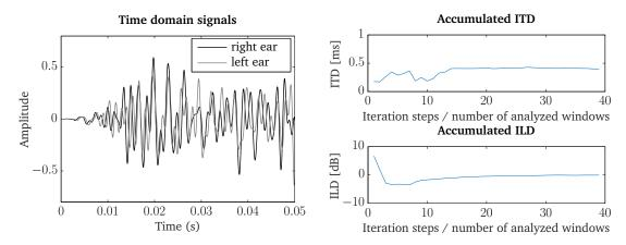
**Figure 4.23:** Left panel: band-pass input noise signal, 400 ms long (only the first 50 ms is shown), 800 Hz wide, centered at 500 Hz, mixed with a reflection of a 2-ms delay, and made binaural with an ITD of 0.4 ms and ILD of 0 dB. Right panel: estimated ITD ILD shown as a function of time frames.
