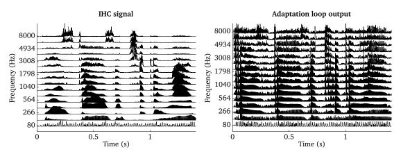
Figure 4.6: Illustration of the adaptation processor. IHC output (left panel) as the input to the adaptation processor and the corresponding output using adpt\_model='adt\_dau' (right panel).
