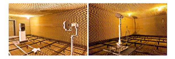
Three-dimensional HRIR datasets were measured with the Neumann KU100 dummy head. An active 3-way louspeaker (Genelec 8260A) was used as a sound source with a constant distance of approximately 3.25m. Different apparent source positions were realized by rotating the dummy head around two axis using the VariSphear measurement system [26]. The impulse responses were captured for different sampling configurations of the source's position:
