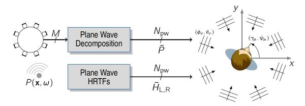
Figure 3.3: Data-based binaural synthesis including small scale translatory movements of the listener. The number of microphones is denoted by M, the number of plane waves by  $N_{\rm pw}$ , the coefficients of the plane wave decomposition by  $\bar{P}$ , the left/right far-field HRTFs by  $\bar{H}_{\rm L,R}$ . The incidence angles of the plane waves is denoted by  $(\phi_{\nu}, \theta_{\nu})$ , the look directions of the listener by  $(\gamma_{\mu}, \psi_{\mu})$ .
