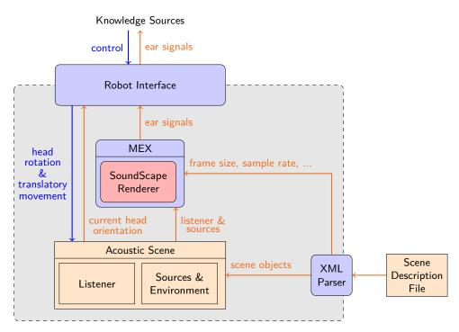
Figure 3.4: Software architecture of the binaural simulator
