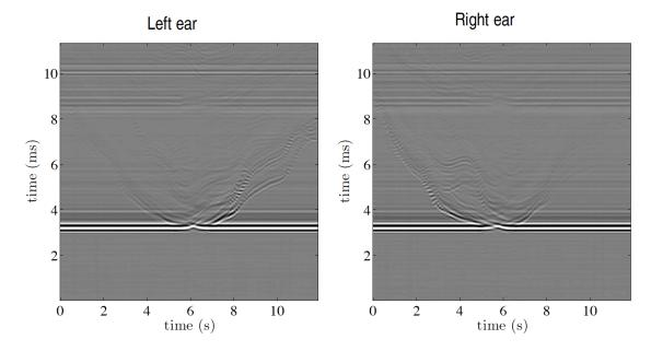
**Figure 3.2:** Dynamic BRIRs captured in a typical office room using a static loudspeaker and HATS position. The horizontal axis denotes the time t at which a BRIR has been captured. The vertical axis shows the time axis  $\tau$  of the BRIR. A vertical slice represents a BRIR at a given time. A moving scatterer is obstructing the direct path between loudspeaker and HATS at  $t \approx 6$  s.
