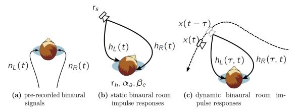
**Figure 3.1:** Techniques for binaural synthesis applied in Two!EARS. Left/right binaural signals are denoted by  $n_{\{L,R\}}(t)$ , BRIRs by  $h_{\{L,R\}}(t)$ , time-variant BRIRs by  $h_{\{L,R\}}(\tau,t)$ . The source signal is denoted by x(t), the source and receiver position by  $r_s$  and  $r_h$ , respectively.
