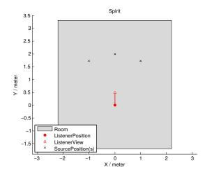
The BRIRs are measured with the same hardware involved in database entry #13. The measurements were done with three loudspeakers placed at different positions and head rotations from  $-90^{\circ}$  to  $90^{\circ}$  with a resolution of  $1^{\circ}$ .
