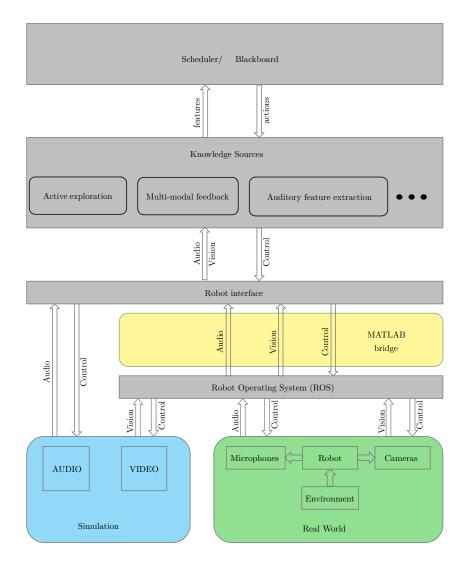
Figure 2.1: Architecture of audio-visual simulation framework.
